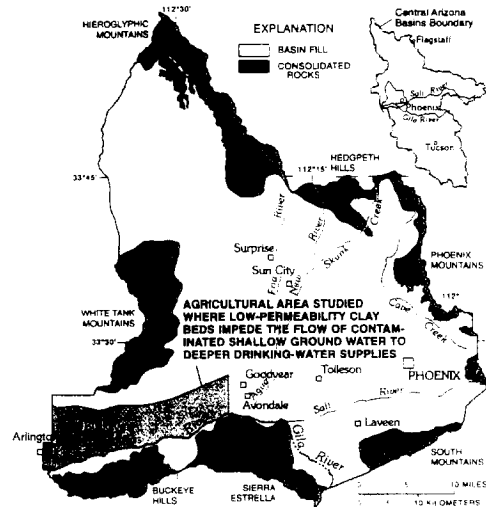
Figure 20. Low-permeability clay beds in an agricultural area in the West Salt River Valley reduce the likelihood of contamination reaching deeper drinking-water supplies.
